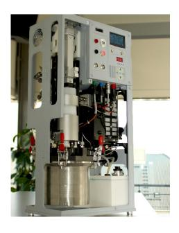
Picture 2: TRL 5 demonstrator of a power generator with a POWERPASTE cartridge and a 100 watt PEM fuel cell.
