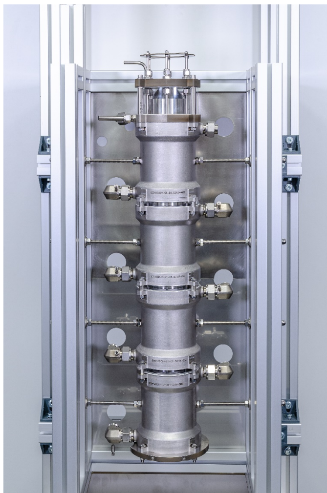
Picture 3: Modular pilot plant for synthesis of Grignard reagents, featuring a maximum throughput of 20 L/h.
