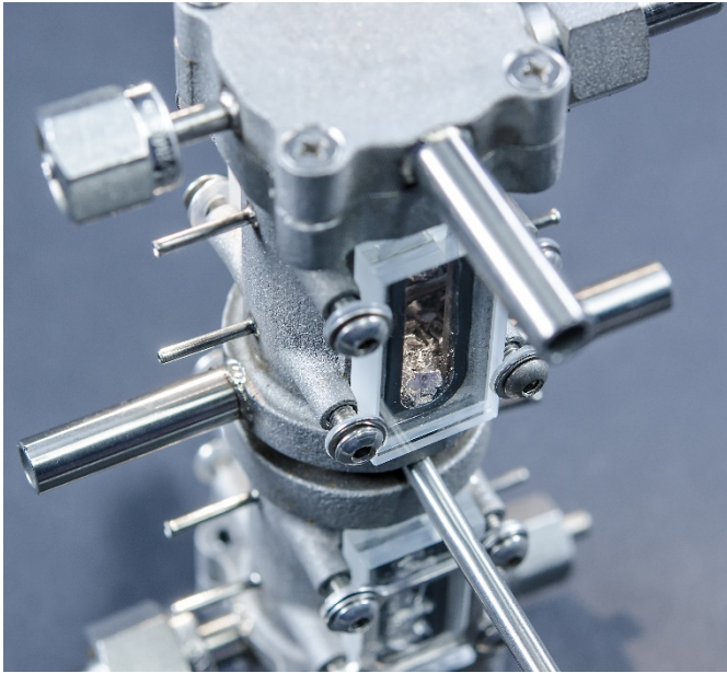
Picture 1: View of the lab reactor for synthesis of Grignard reagents.
