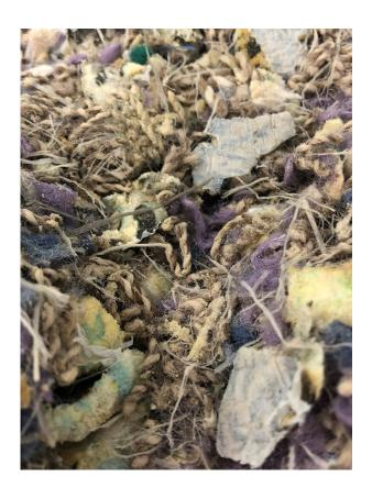
Picture 2 Broken-down carpet waste that is subsequently cleaned and has ionic liquid added to it.
