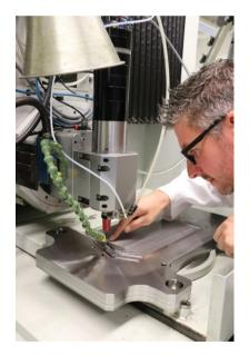
Fig. 2 Udo Eckert, Group Leader Microsystems Manufacturing & Technical from the Functional Surfaces and Micromanufacturing department at Fraunhofer IWU, tests the finishing of a milled tool to be used in bipolar plate production for fuel cells at the micromachining center of Fraunhofer IWU.
