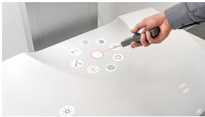
The Multimodal Dialog Assistant for manual quality control in industry can be controlled by voice or gestures. (© Fraunhofer CCIT/Fraunhofer IAIS)
