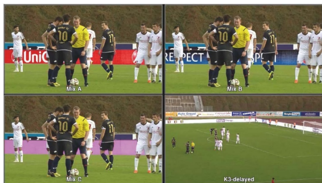
Picture 2: Soccer players in front of LED boards: The magenta-colored surface only appears for 2 milliseconds and is invisible to both spectators in the stadium and TV viewers. They only see the advertising that is intended for them.
