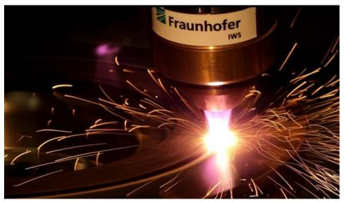
HICLAD enables high-quality corrosion coatings in an efficient process. © Fraunhofer IWS Dresden
