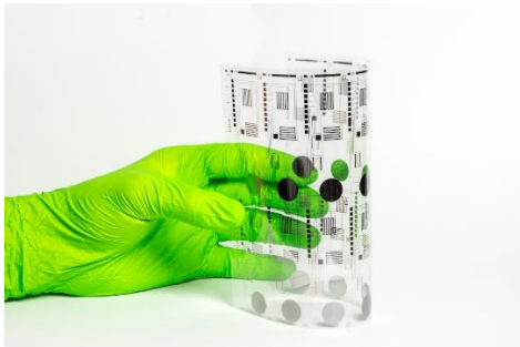
Fig. 1.: Printed functionalities on a flexible polymer foil for covering microfluidic chips.
