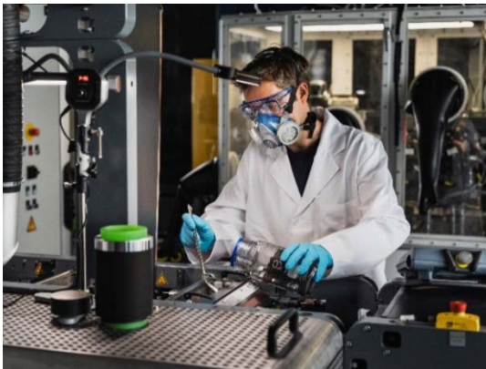
Fig. 1 The dry coating powder is fed into the calender gap in the DRYtraec® machine.
