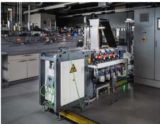
Fig. 3 DRYtraec® machines do not require long drying tracks and so take up significantly less space than conventional battery electrode manufacturing systems.
