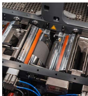
Fig. 2 A fine coating film forms on the faster-rotating roller.
