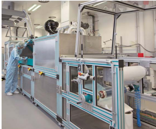
Fig. 3 The coatings are manufactured using a roll-to-roll process. At just a few hundred micrometers thick, both the electrochromic film and the thermochromic thin glass substrate are extremely thin.
