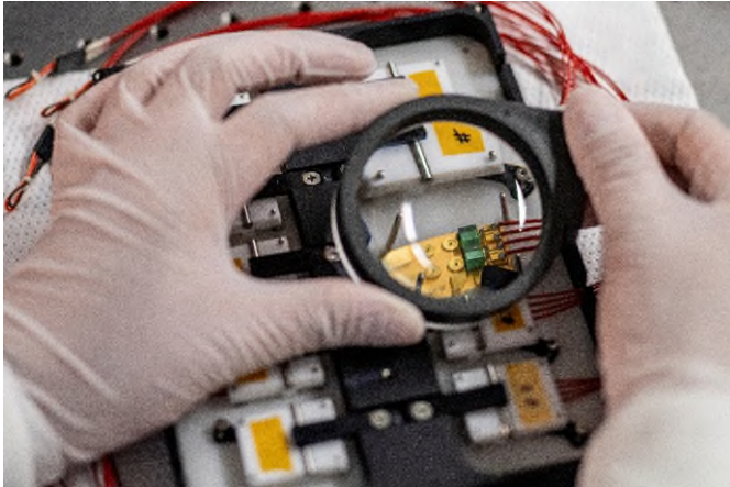
Picture 2 Raman spectrometer the size of a 50-cent piece.
