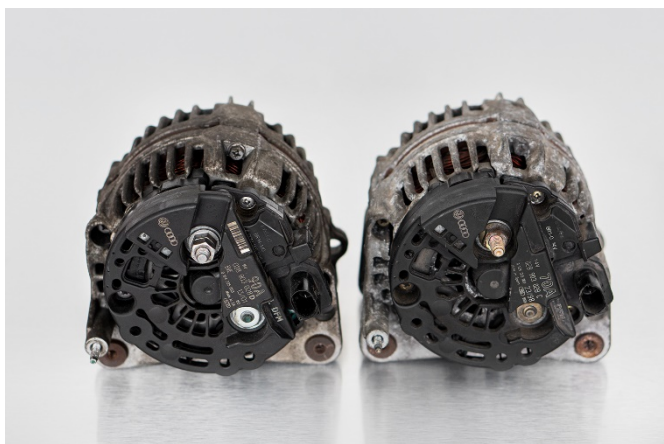
Picture 2 Product variance – two generators with different part numbers are visually identical.
