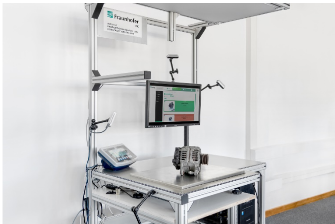
Picture 1 AI-supported assistance system for semi-automated sorting of used components.
