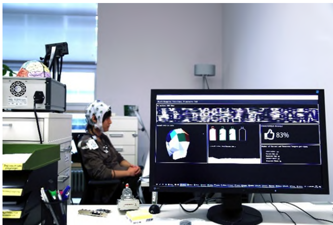
Fig. 3 In practical testing, the research team uses multimodal neurophysiological and psychophysiological measurement procedures as well as machine learning methods to find out how much emotional and cognitive processes the subject is under – for example, when operating a software program.
