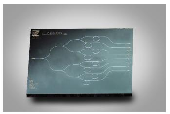
One of the photonic sensor chips developed as part of the optION project with eight sensor channels made from silicon nitride.
