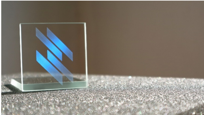
Picture 2 Laser-functionalized glass with decorative Fusion Bionic logo inspired by the morpho butterfly.
