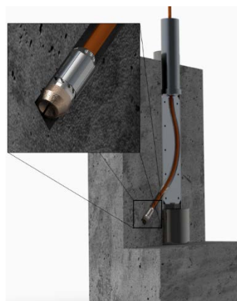
Fig. 2 Simple and reliable: the sheet steel deflection shoe guides the drilling tool outward at an angle of 45 degrees.
