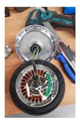
Fig. 2 The electric motor in an e-scooter is in the tires: The magnets are the silver cuboids on the edge of the copper coils.
