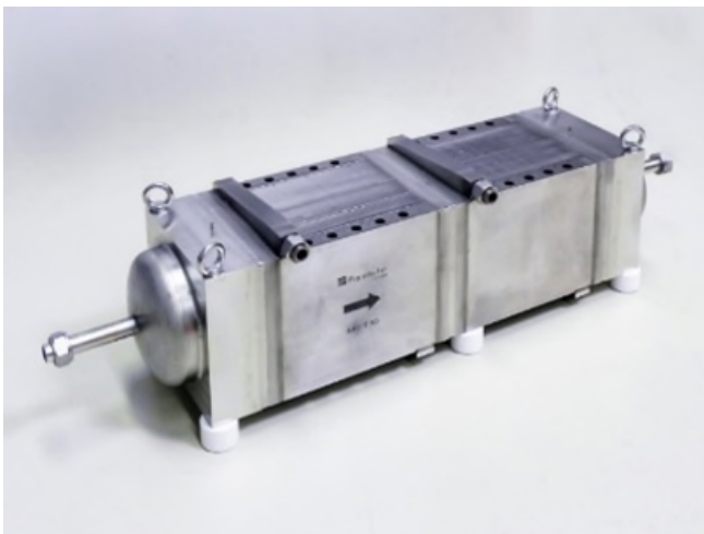
Fig. 1 Reactor for catalytic methanation of CO 2 , 50 kW nominal output.
