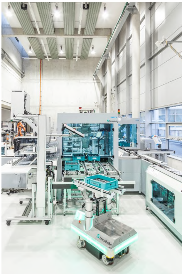
Fig. 2 Autonomous robots working as temporary storage during production.
