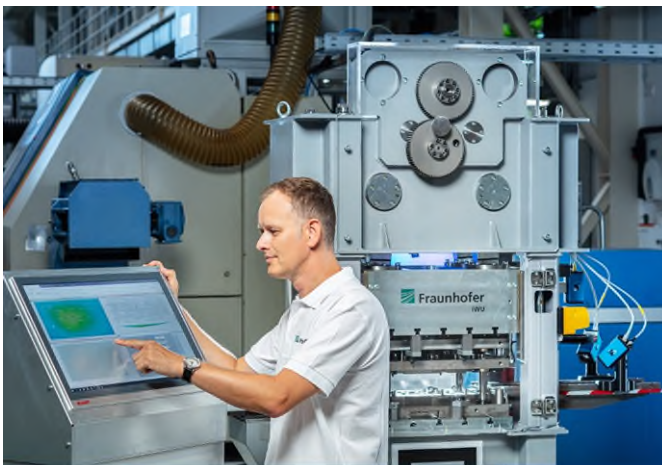
Fig. 1 A forming press demonstrator provides visitors with live insights into how a cognitive T-slot works. The process data transferred by smartNOTCH is visualized on a connected terminal.
