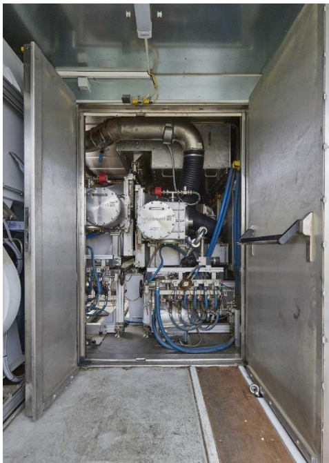
The truck-based mobile system can treat 25 tons of seed per hour.
