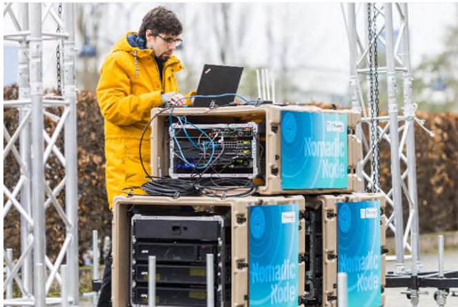
Fig. 1 The entire hardware and software for the 5G+ Nomadic Node fits into a couple of mobile server rack containers.
