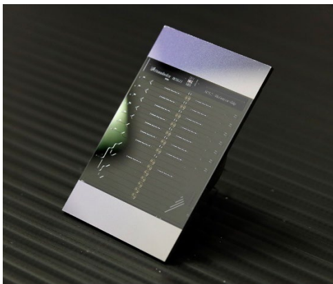
Picture 1 Integrated waveguides in silicon technology fabricated on 200-mm silicon wafers and used in combination with a functionalized surface as highly sensitive biosensors.
