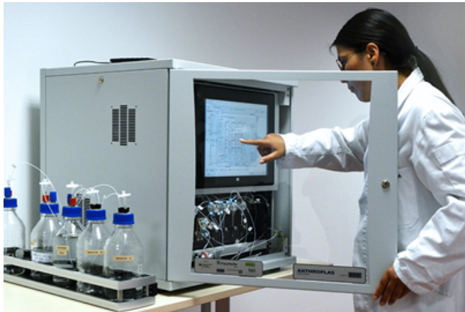
Fig. 2 An optical sensor system that detects micro-pollutants in wastewater. In the future, the system will be able to control purification processes in line with demand.
