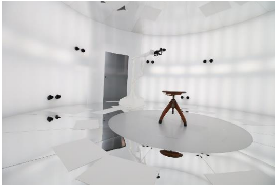
Fig. 1 The rotunda is equipped with 32 cameras that film the lecturer from all sides. A lifelike 3D avatar is generated from the video data.
