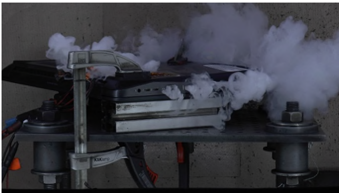
Fig. 1 Gas being emitted from a laptop battery during thermal runaway
