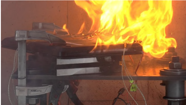
Fig. 2 A laptop on fire during thermal runaway
