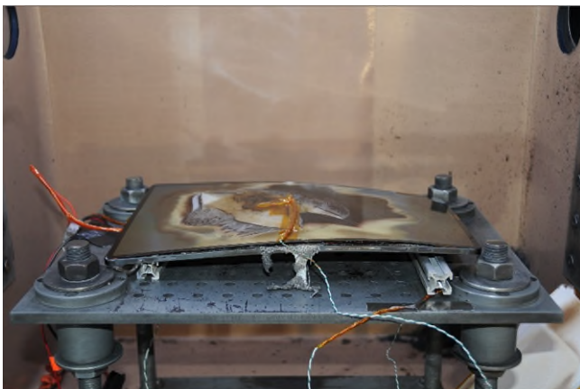
Fig. 3 A tablet destroyed after thermal runaway
