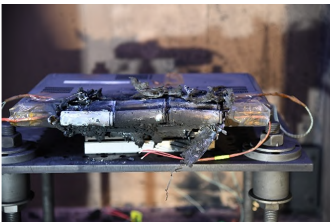
Fig. 4 A laptop destroyed after thermal runaway
