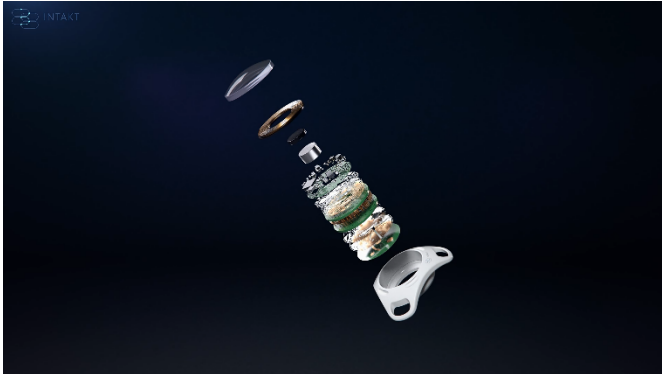
Fig. 2 Complex functionality in a tiny capsule: The microimplant consists of an eight-layer circuit board.
