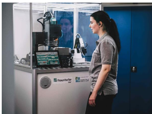
Fig. 1 Machines such as this milling machining center can be controlled using speech recognition systems and audio technology from Fraunhofer IDMT in Oldenburg. This reliable system can be quickly and easily adapted to customers’ needs.
