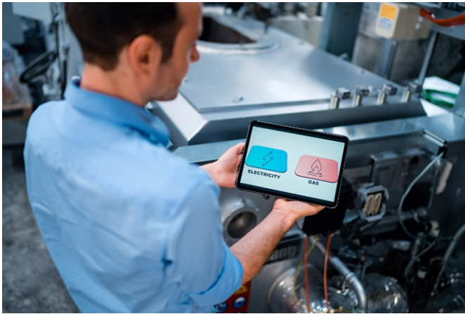
Abb. 2 Bivalent crucible furnaces can switch dynamically between electricity and gas during operation.
