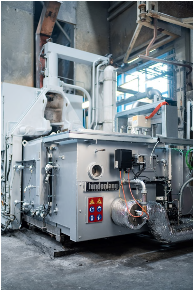
Abb. 1 Energy flexibility during production: Bivalent crucible furnaces can switch energy usage to the power grid without affecting production.
