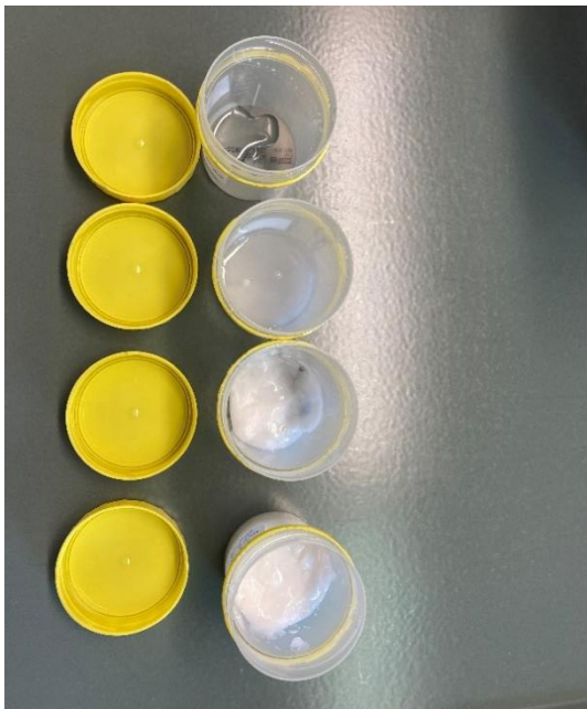
Fig. 1 Cyclodextrine gels as adsorber material enclose the toxic wood preservatives and completely encapsulate them.
