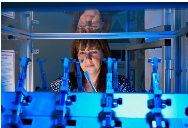
Fig. 2 Daily mechanical teeth cleaning was replicated in a toothbrushing simulator during the in-vitro study.
