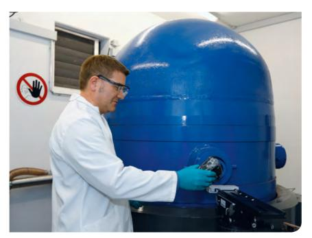
Unused explosives are disposed of in a detonation chamber weighing 20 metric tons.
