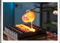
Casting and cooling the molten glass in graphite molds.
