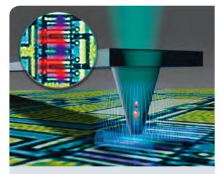
Schematic representation of a scanning probe quantum magnetometer with an NV diamond tip that provides an image-based representation of the currents in a nanoelectronic circuit. © *Fraunhofer IAF*
