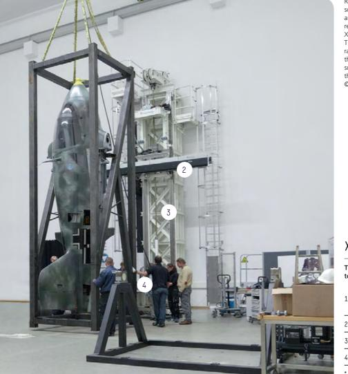
Reims and his team scanned the aircraft in an upright position, thus reducing the distance the X-rays had to penetrate. This ensured that more radiation reached the detector, thereby substantially improving the quality of the scan. © Fraunhofer IIS
