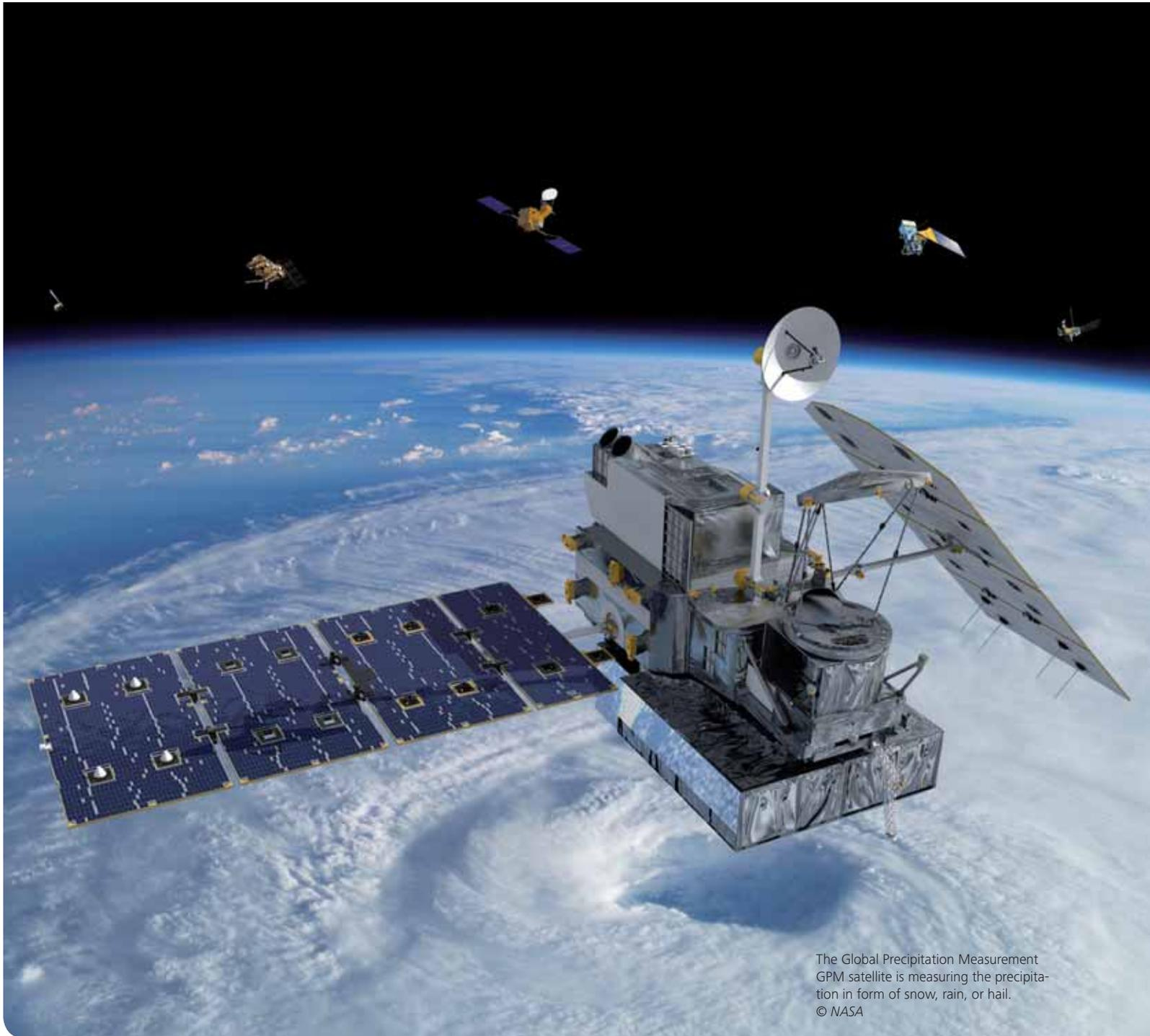
The Global Precipitation Measurement GPM satellite is measuring the precipitation in form of snow, rain, or hail.
