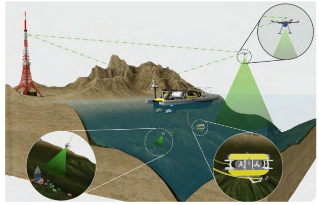
The SeaClear clean-up fleet consists of an autonomous mother ship with collection containers on the surface, a drone flying in the air and two underwater robots, with one finding and the other gathering the waste. © *S. Sosnowski* – *SeaClear Project*
