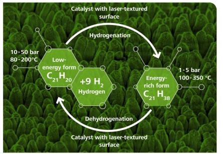
Laser texturing to the surface of a metal catalyst enlarges its area, thereby enhancing the efficiency of the reaction to produce liquid organic hydrogen carriers (LOHCs). When bound in this form, hydrogen can be stored without hazard. Source: Fraunhofer HHI © *Graphics: Vierthaler & Braun*
