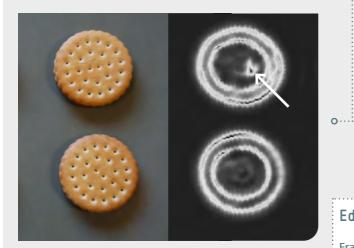
A radar image clearly reveals the presence of glass splinters in the filling of a chocolate cream cookie. © *Fraunhofer FHR*
