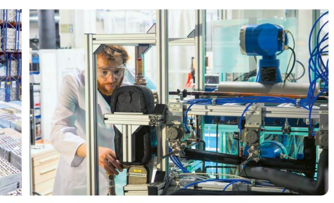
Clemens Dankwerth from Fraunhofer ISE examines a propane refrigeration circuit for leaks in the test laboratory. The refrigeration circuit is one of the central components of the newly developed LC 150 heat pump, which works with propane as its environmentally friendly refrigerant. © Fraunhofer ISE/Marek Miara
