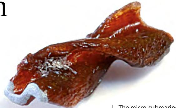
The micro-submarine is steered via a neodymium-iron-boron tip.
