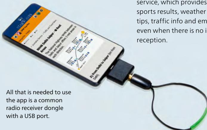
All that is needed to use the app is a common radio receiver dongle with a USB port.
