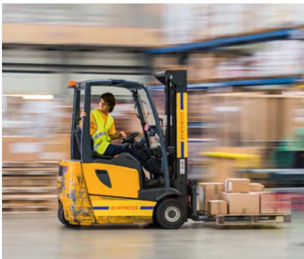
Forklifts travel at 6 to 7 kilometers per hour and may have an unladen weight of over 500 kilograms.
