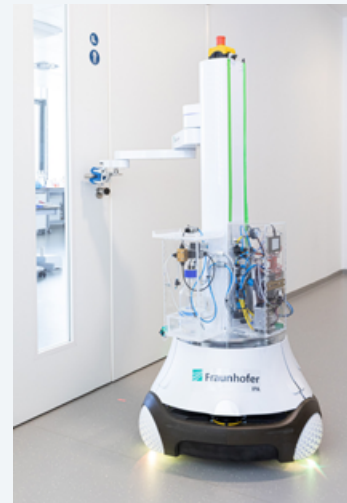
The DeKonBot independently disinfects objects such as door handles.
