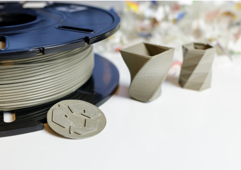
Prepared material for additive manufacturing: Post-consumer waste is processed into filaments for 3D printing. Photo: Fraunhofer IFAM
