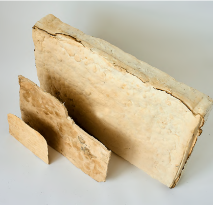
Flexible mycelium materials in different thicknesses can be used as upholstery material, insulation board or alternatives to leather. Photo: Fraunhofer IAP / Jadwiga Galties
