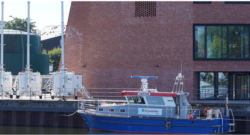
KIRMES deploys a mobile infrastructure for data collection with a sensor network comprising three Cells on Wheels and a research vessel. Photo: Fraunhofer CML
