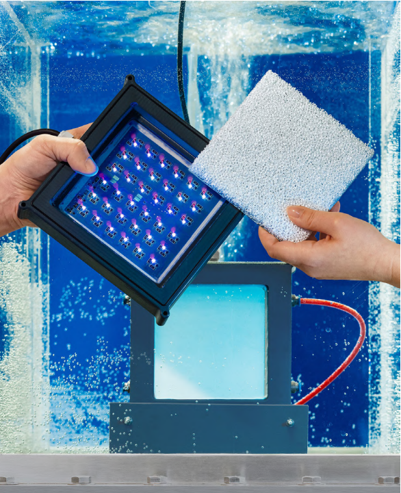
Ceramic stack system with multifunctional ceramic foam and LED array for efficient photocatalytic treatment of industrial process water and wastewater. Photo: Fraunhofer IKTS
