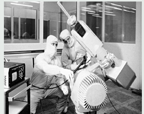
An industrial robot being tested for compliance with clean-room specifications.
