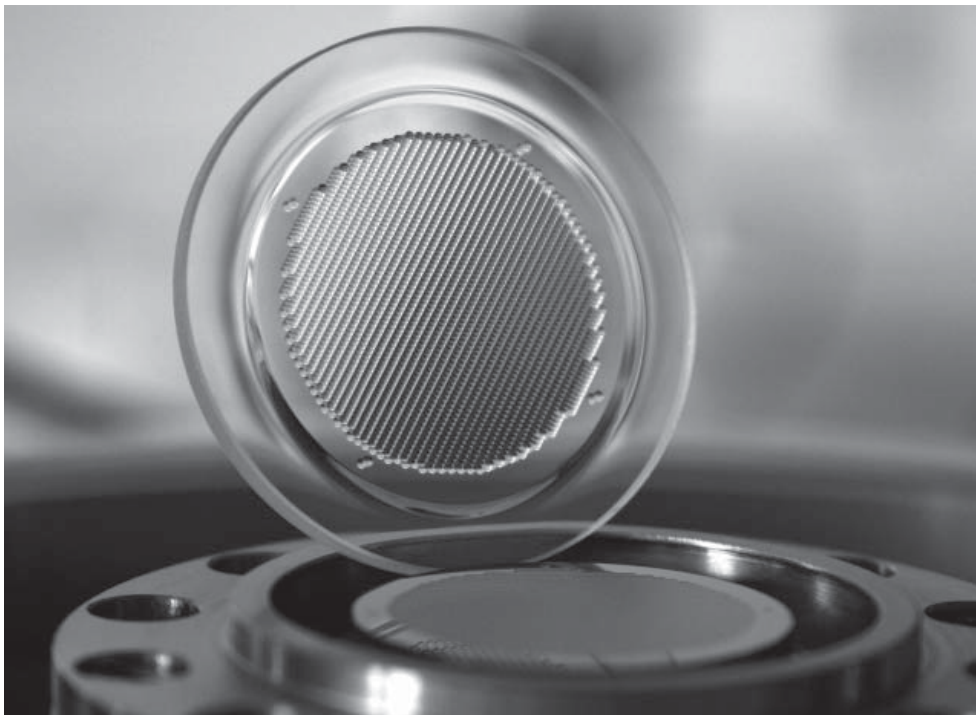
The finished lens array is at a slant behind the lower die set of the hot embossing equipment. (© Fraunhofer IWU)
