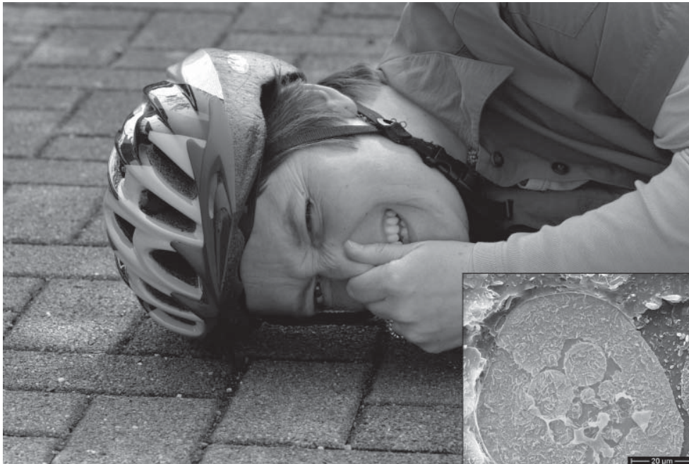
The damaged helmet releases odoriferous substances. Bottom right: the opened microcapsule. (© Fraunhofer IWM)
