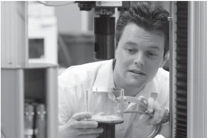
A researcher installs an environmental chamber in the special laboratory in which metals' susceptibility to stress corrosion can be tested. (© Fraunhofer IWM)
