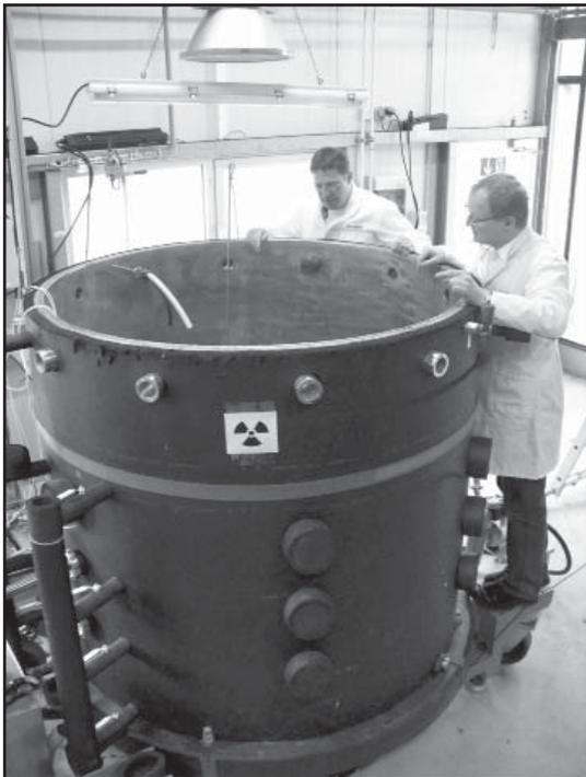
Researchers inspect the two-cubic-meter water tanks equipped with a powerful filter system.
