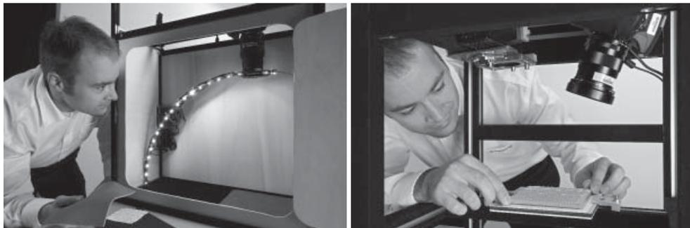
The HDR-ABTF scanner captures physically realistic images of materials such as textiles, lit from various different angles (left). The meso scanner records detailed 3-D structures of surfaces with great precision (right). (© Fraunhofer IGD)
