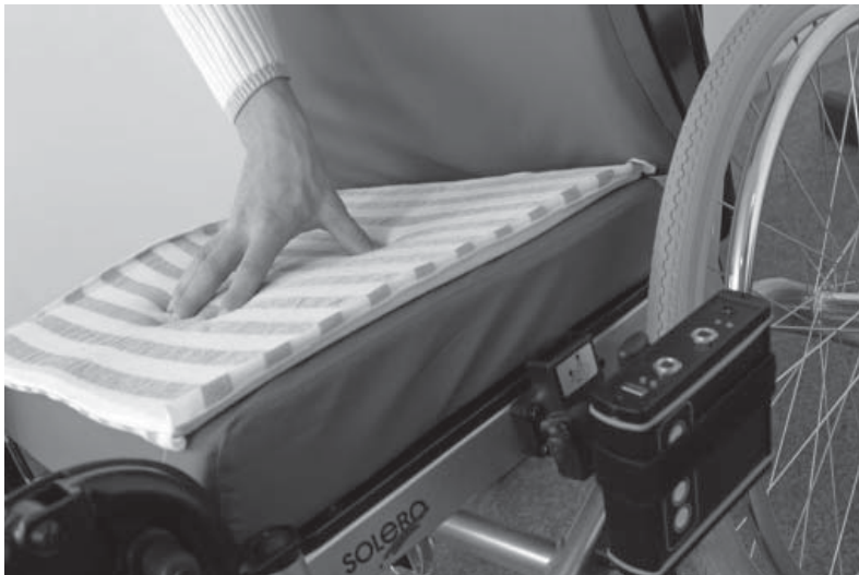
A sensor mat integrated in a wheelchair set helps prevent pressure ulcers. (© Fraunhofer IFF)
