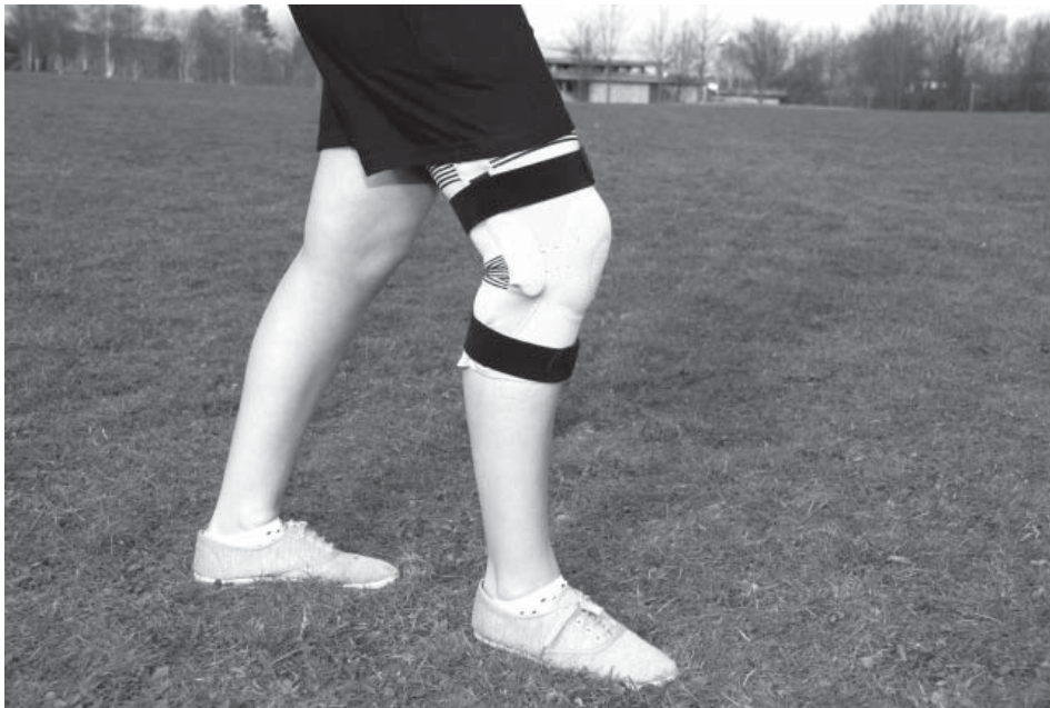
Sensors integrated into the bandage register the knee's range of movement. (© Fraunhofer IPA)
