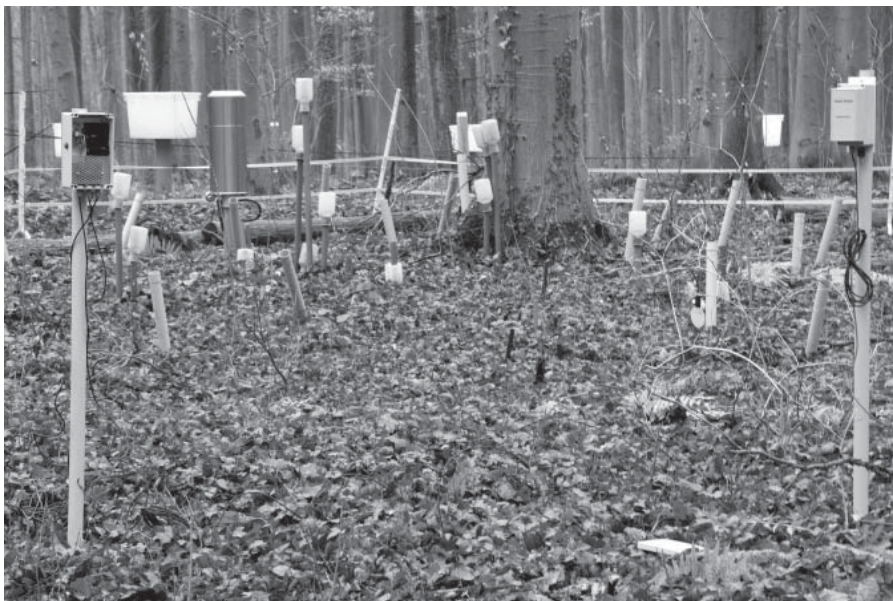
A wireless sensor network records data such as soil and leaf humidity, as well as air temperature. (© Fraunhofer IMS)
