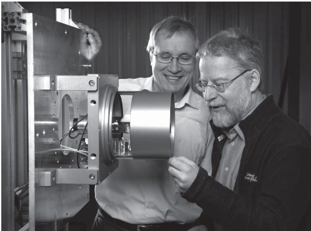
Dr. Heinrich Höfler and Dipl.-Ing. Harald Wölfelschneider (from left to right) with a 3D laser scanner that improves safety and reliability on railroad tracks all over the world.
