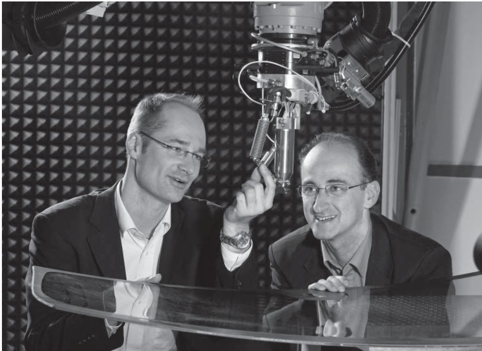
Dr. Jörg Ihde and Dr. Uwe Lommatzsch (from left to right) have developed a new coating process for functional nano-layers, using a plasma nozzle that works at atmospheric pressure. (© Dirk Mahler/Fraunhofer) | Picture in color and printing quality: www.fraunhofer.de/press
