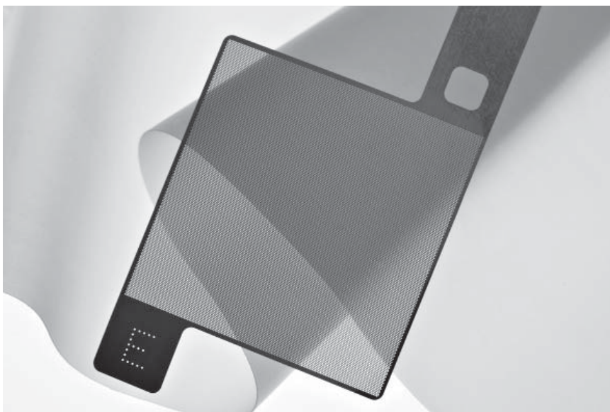
This image shows the lattice-shaped electrode in the foreground, and the elastomer in the background. (© Ursula Raapke) | Picture in color and printing quality: www.fraunhofer.de/press
