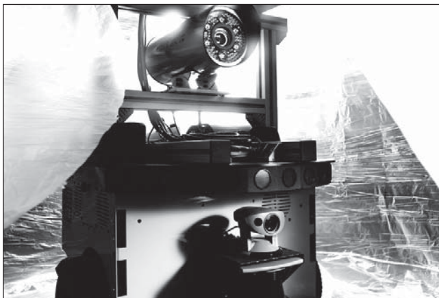
Equipped with multiple sensors and optical cameras, the mobile robot roams over dangerous ground. (© Fraunhofer IOSB)
