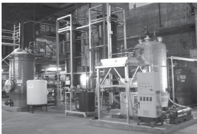
This plant in Stuttgart makes biogas out of waste from wholesale markets. (© Fraunhofer IGB)
